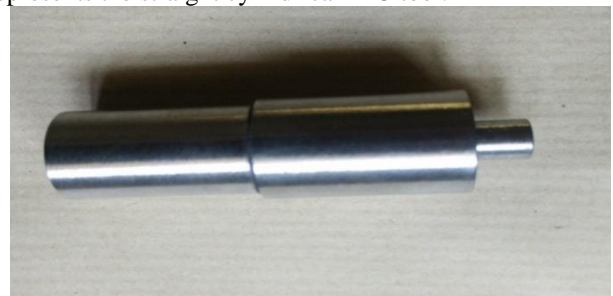
Fig. 1: Straight cylindrical H13 tool
