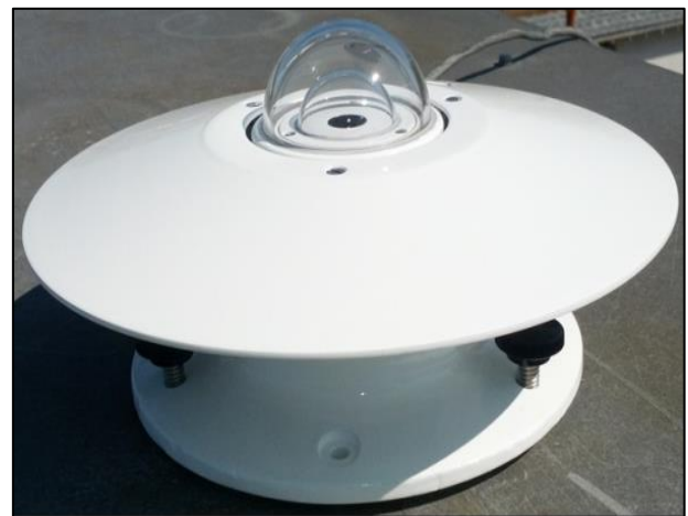
Fig. 9: Eppley precision pyranometer ( http://www.eppleylab.com )
