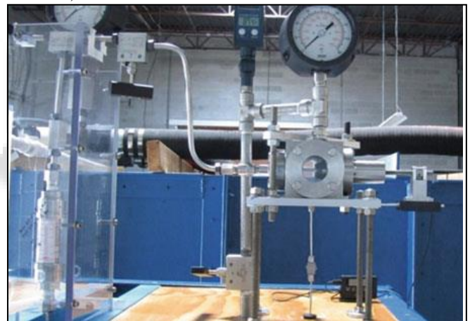
Fig. 2.6 Picture of the G134 “7 ksi (48 MPa) - 5 gpm (0.3 l/s)” test chamber loop
