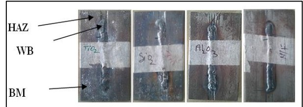
Fig. 2: Photographic View of Sample after Welding of Mild Steel
