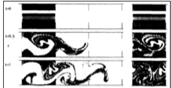
Fig. 3: Results for a baffled channel with no oscillatory component in the flow at Re = 300 . [9]
