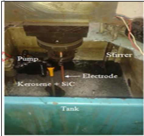
Fig. 2: PM- EDM Setup used for Experimental Work
