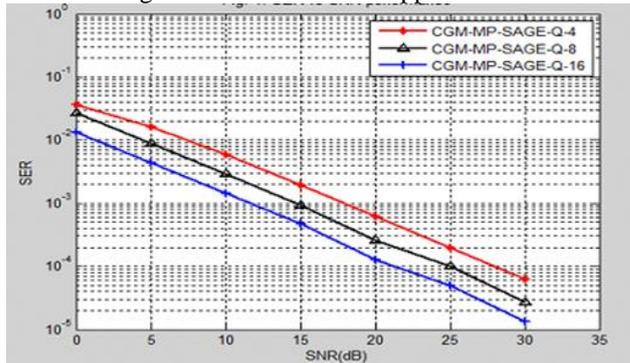
Fig. 6: SER vs SNR performance of CGM-MP-SAGE algorithm for different resolution factors.
