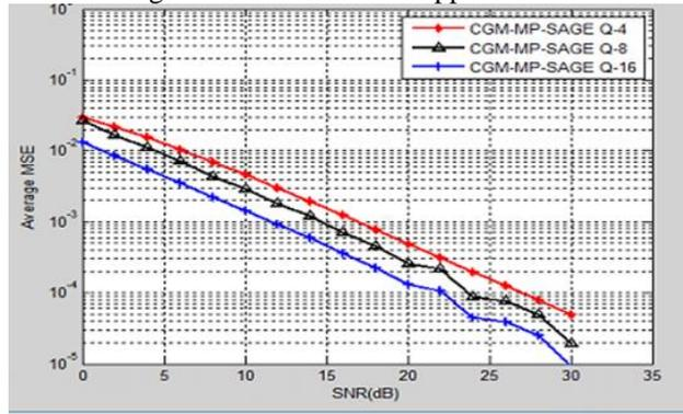
Fig. 10: MSE vs SNR performance of CGM-MP-SAGE algorithm for different resolution factors.
