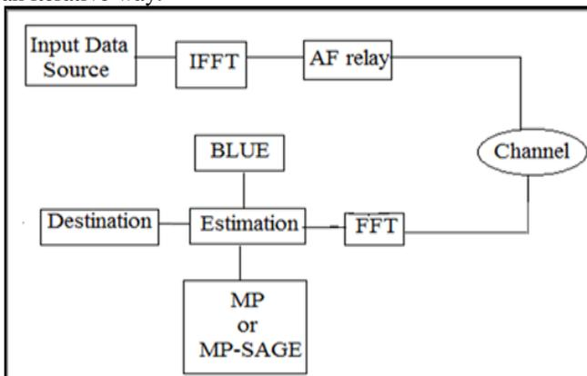
Fig. 2: Block diagram of channel estimation.
