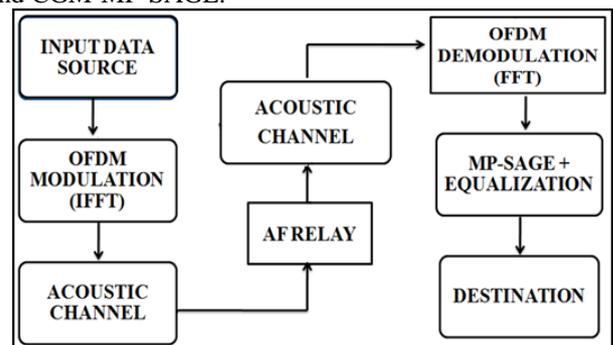
Fig. 3: Designed system block diagram
