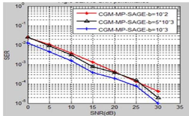
Fig. 5: SER vs SNR performance of the CGM-MP-SAGE algorithm for different Doppler rates.
