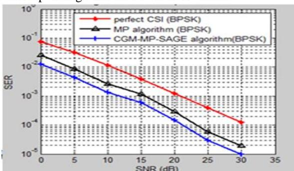
Fig. 4: SER vs SNR performance, BPSK comparison perfect CSI, MP and CGM-MP-SAGE algorithm
