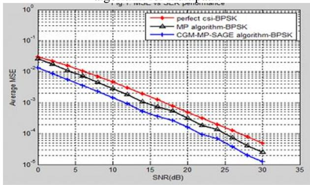
Fig. 8: MSE vs SNR performance, BPSK comparison perfect CSI, MP and CGM-MP-SAGE algorithm.
