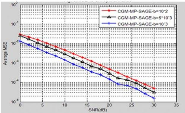
Fig. 9: MSE vs SNR performance of the CGM-MP-SAGE algorithm for different Doppler rates.
