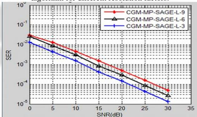
Fig. 7: SER vs SNR performance of CGM-MP-SAGE algorithm for multipath.
