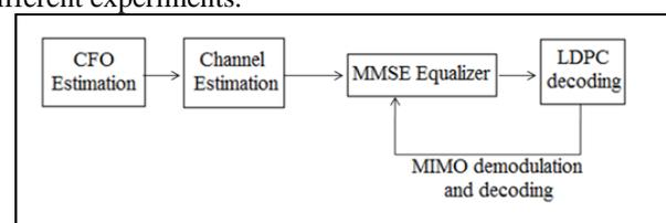
Fig. 1: Receiver block diagram
