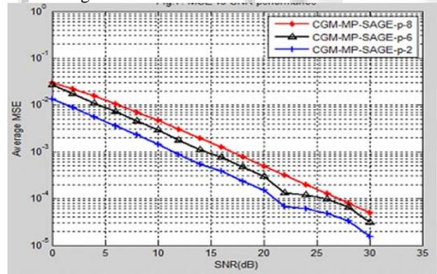
Fig. 11: MSE vs SNR performance of CGM-MP-SAGE algorithm for different pilot spacing
