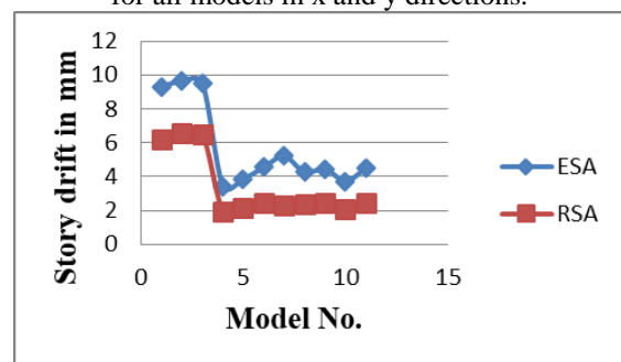
Fig. 5: Storey Drift vs. Model for Different Models along X-Direction by ESA and RSA
