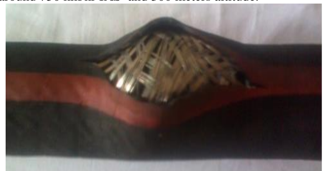
Fig. 1: Close –up photograph of the damaged - area of the mid-air refuelling hose.
