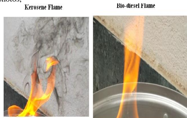
Fig. 1: comparison of flames of kerosene and biodiesel
