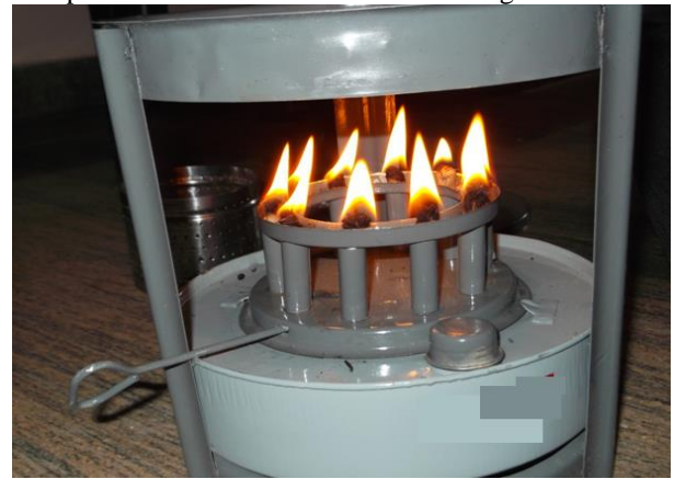
Fig. 8: Result of biodiesel wick stove
