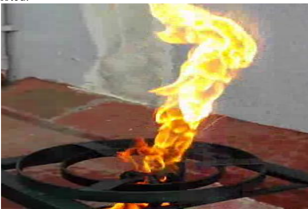
Fig. 7: Result of gravity fed biodiesel stove
