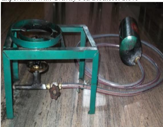
Fig. 7: Gravity fed biodiesel stove
