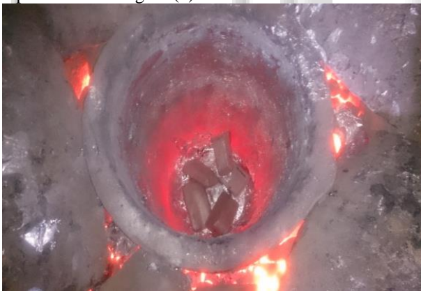
Fig. 2: Melting of Al2024 metal in furnace.
