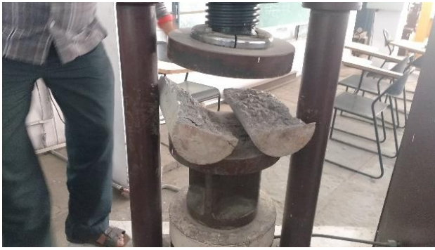
Fig. 5: Specimens tested for Split Tensile Strength for 7 Days and 28 Days
