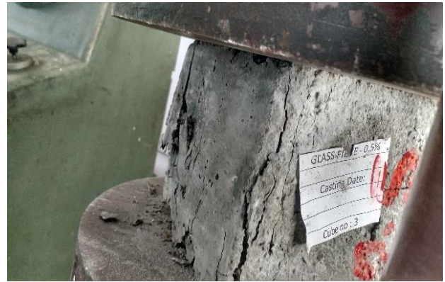
Fig. 3: Specimens tested for compressive strength for 7 Days and 28 Days
