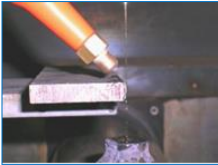
Fig. 1: EDM Process Set-up
