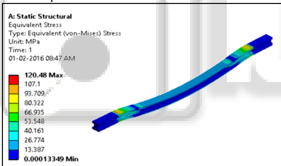
Fig. 29: Stress Report for I-Section Axle
