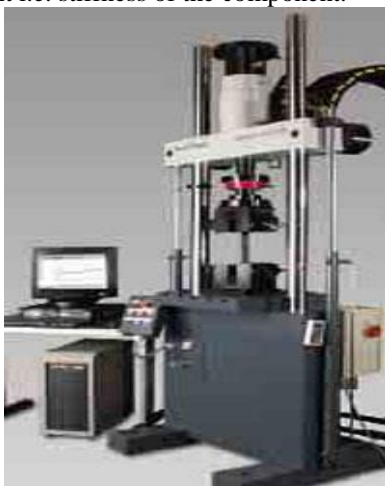
Fig. 8: Typical test setup for physical experimentation to calculate stiffness
