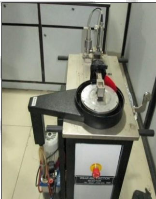
Fig. 1: Wear and friction monitor machine [16] .
