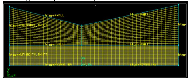
Fig. 4: CD-2, CD Nozzle with presence MDT, with grid points 40X50
