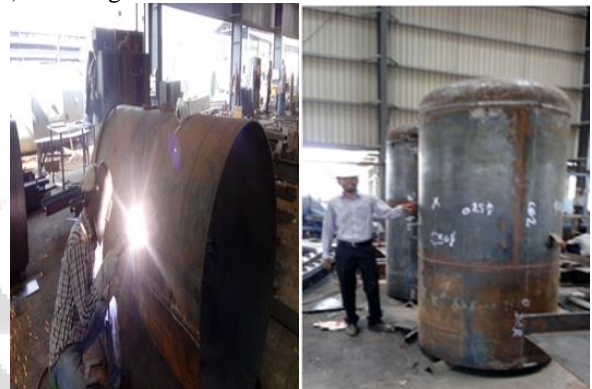
Fig. 10: Final Fabricated Pressure Vessel
