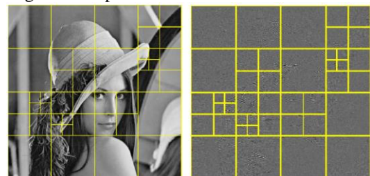
Fig. 2: QTD segmentation into blocks of variable size. (a) Noisy image; (b) Horizontal subband ( HH_1 ) after DWT
