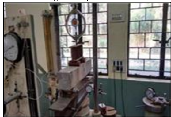
Fig. 5: Composite beam with a two point loading.
