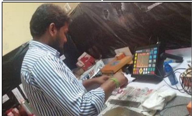
Fig. 4: UFD, TR probe and scanning of samples
