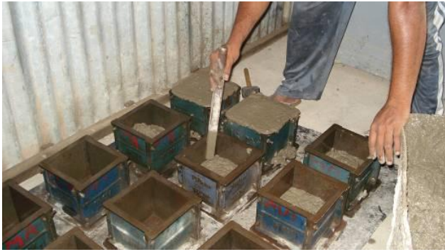
Fig. 3: Casting Of M80 Cubes With Different Water Content
