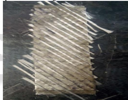
Fig. 2: Fibre at 30° Orientations
