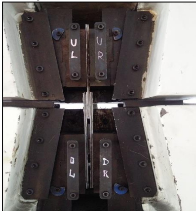
Fig. 8: UTM machine Sample loaded condition for tensile testing
