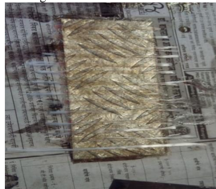
Fig. 3: Fibre at 90° Orientation
