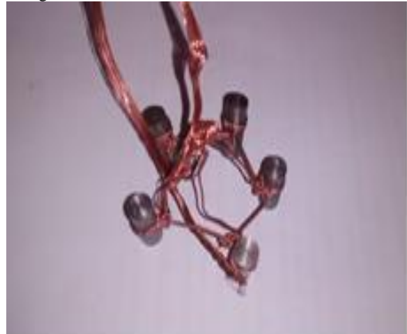
Fig. 3: M S specimens for coating
