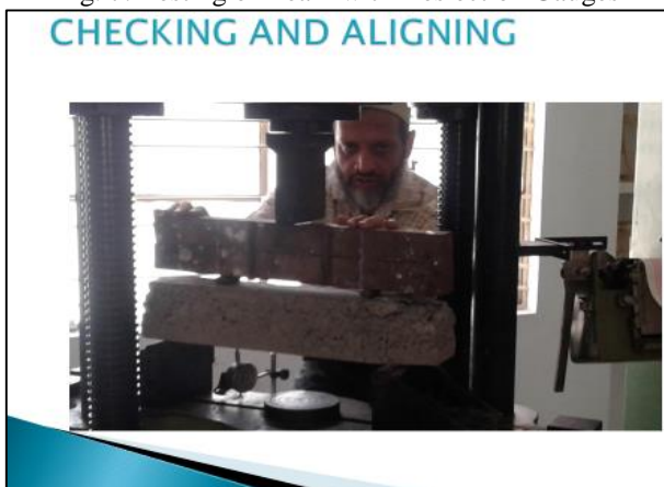
Fig. 8: Checking and Aligning
