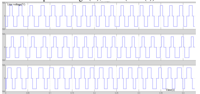
Fig. 10: Line voltage from the stator side Inverter (X-axis: Line voltage (V), Y-axis: Time(s))
