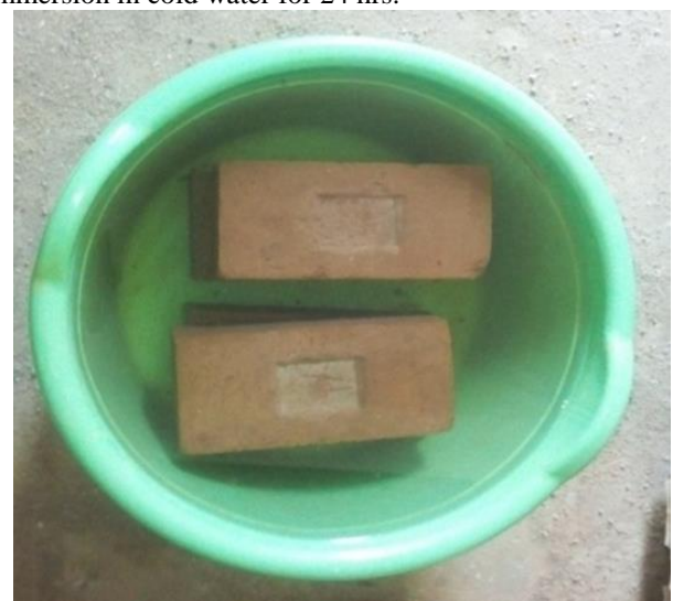
Fig. 6: Water absorption of blocks
