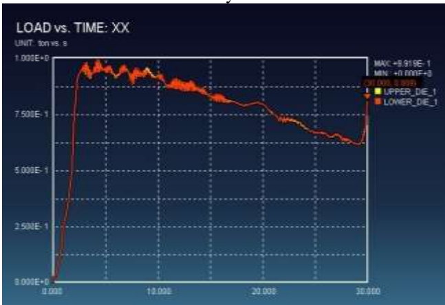
Fig. 8: Graph 2 Die angle-45°, friction co-efficient 0.20 and ram velocity 1.0 mm/s.
