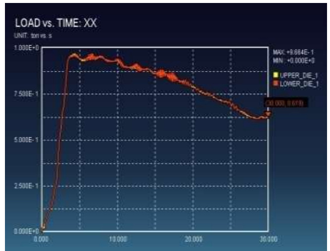
Fig. 9: Graph 3 Die angle-60°, friction co-efficient 0.20 and ram velocity 1.0 mm/s
