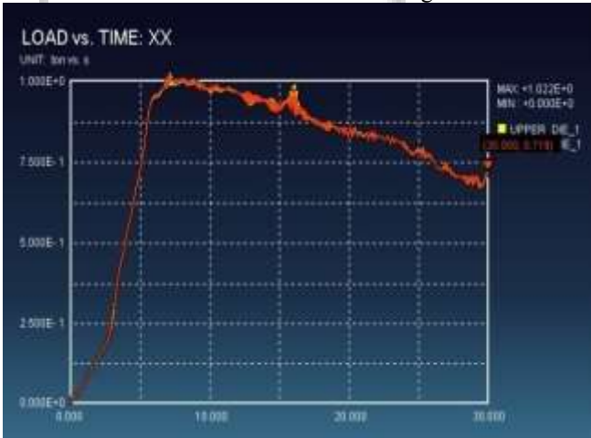
Fig. 7: Graph 1 Die angle-30°, friction co-efficient 0.20 and ram velocity 1.0 mm/s
