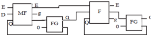
Fig. 11: Master Salve D-FF using MM and F gate
