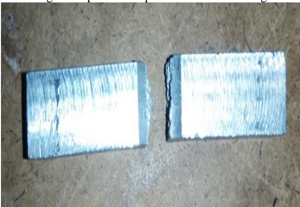
Fig. 5: Impact Test Specimen after Testing
