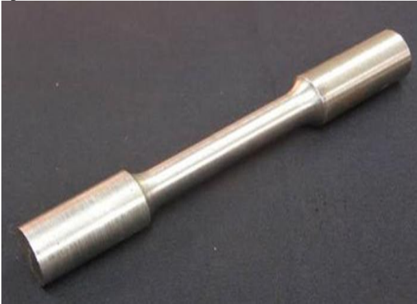
Fig. 2: Tensile Test Specimen Before Testing
