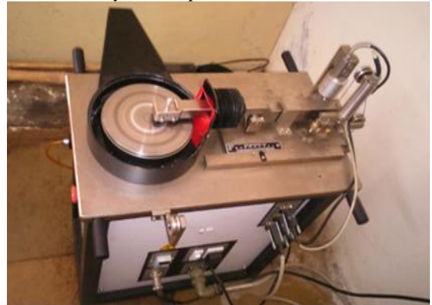
Fig. 15: Pin-on-Disc Wear test set up
