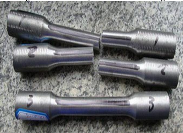
Fig. 3: Tensile Test Specimen after Testing
