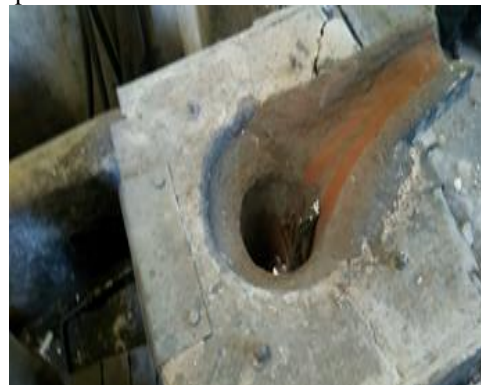
Fig. 1: Induction Furnace with Crucible Containing Al7075
