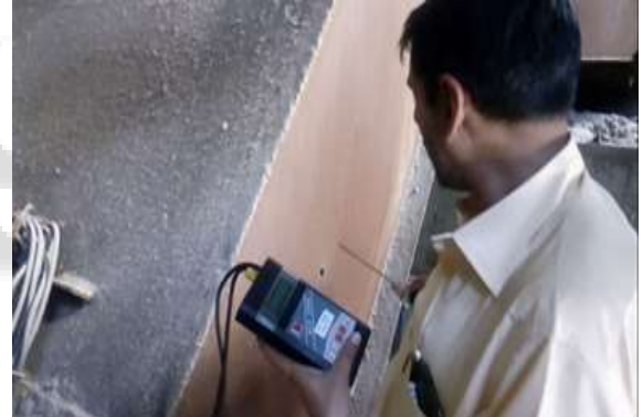
Fig. 1: Flue Gas Analyser Takes Reading At Aph Outlet
