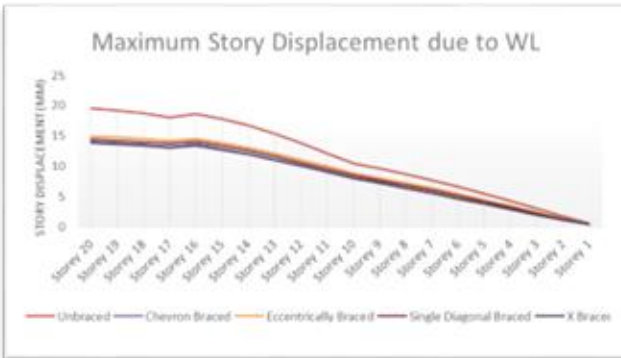
Fig. 15: Storey displacement due to WL
