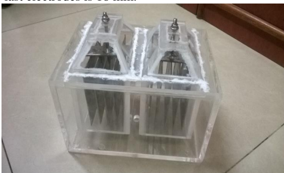
Fig. 1: Design of Electrolyser of A module
