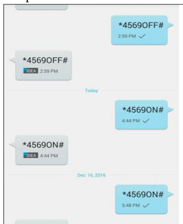
Fig. 3: Result of motor control via SMS
