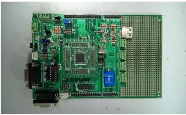
Fig. 2: ARM7 Microcontroller Board
