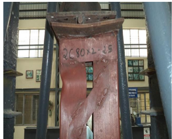
Fig. 9(a), (b): Failure patterns of 2C80x2-25
