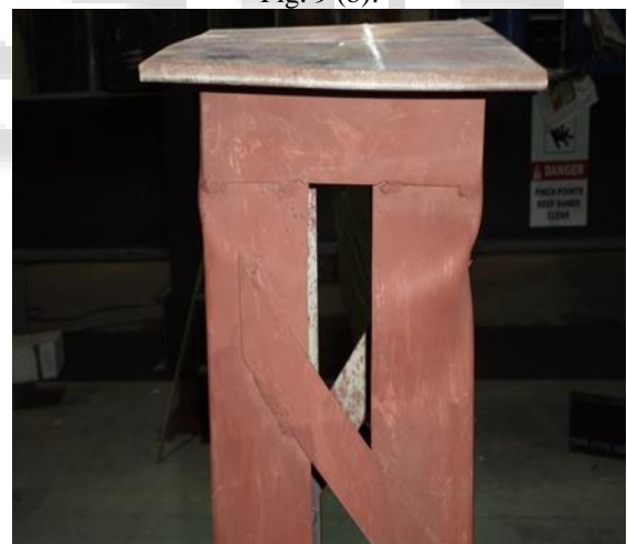
Fig. 10: Failure pattern of 2C80x2-50
