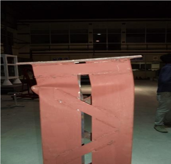
Fig. 11: Failure pattern of 2C100x2-25
