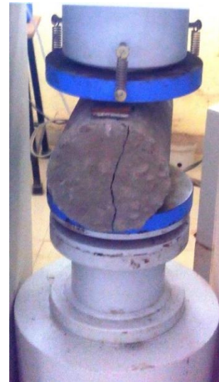
Fig. 2: Split tensile test on Compression testing machine
