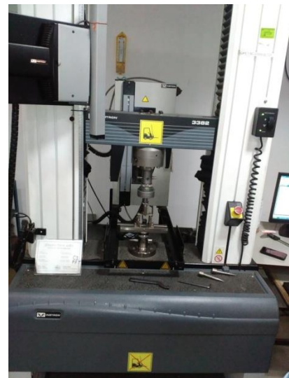
Fig. 2: UTM with flexural test fixture
