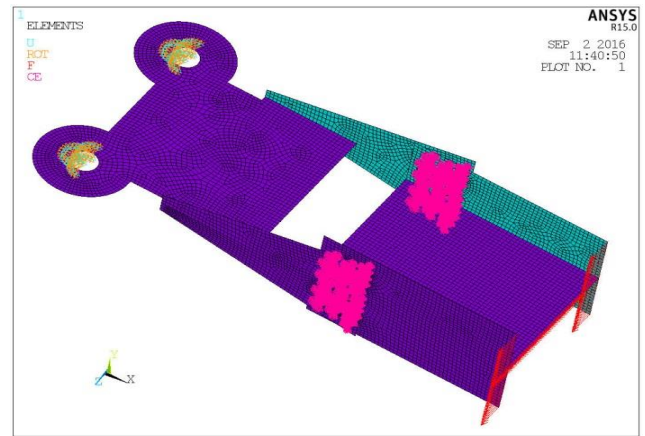
Fig. 9: Boundary conditions used for static analysis
