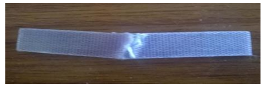
Fig. 14: Impact test specimen after testing
