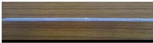
Fig. 9: Flexural test specimen before testing
