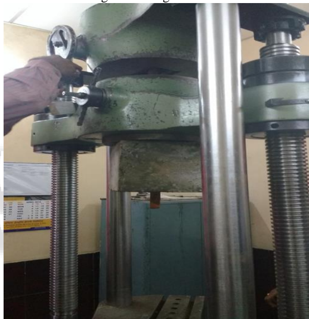
Fig. 6: Testing Of Cube
