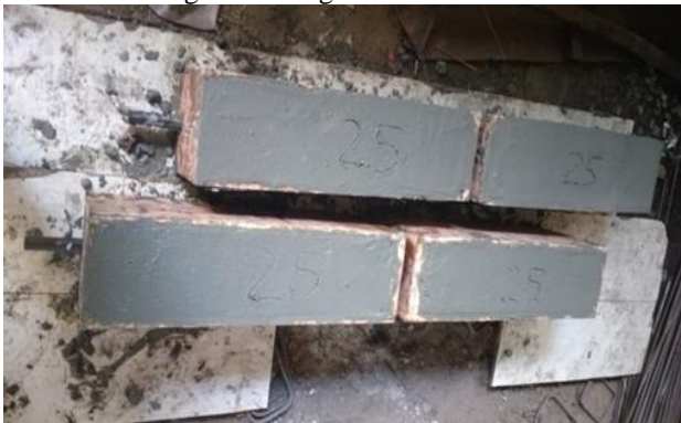
Fig. 3: Casting of M25 Beams
