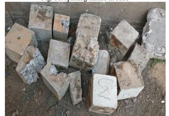
Fig. 17: Failure specimens of pull-out tes
