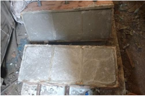
Fig. 2: Casting of Rilem Cubes
