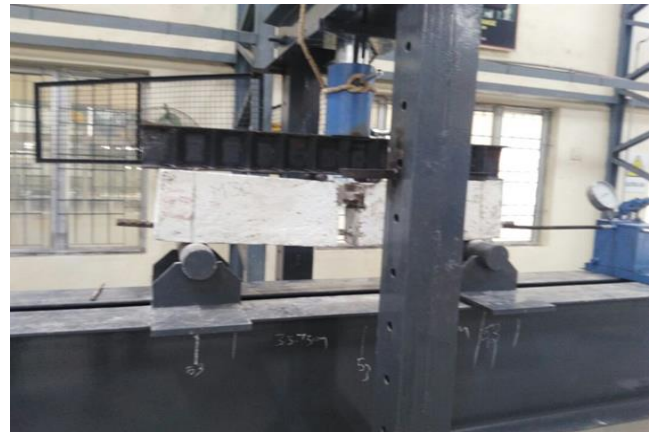
Fig. 14: Failure Pattern -Bending of bar
