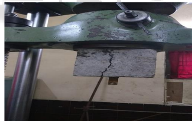
Fig. 16: splitting failure in cube
