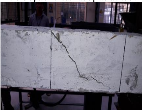
Fig. 8: Failure pattern of SFRC beam
