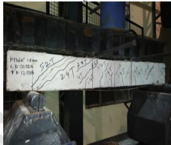
Fig. 6: Typical failure of RC strengthened beam with continuous steel sheet(1.5mm) at bottom
