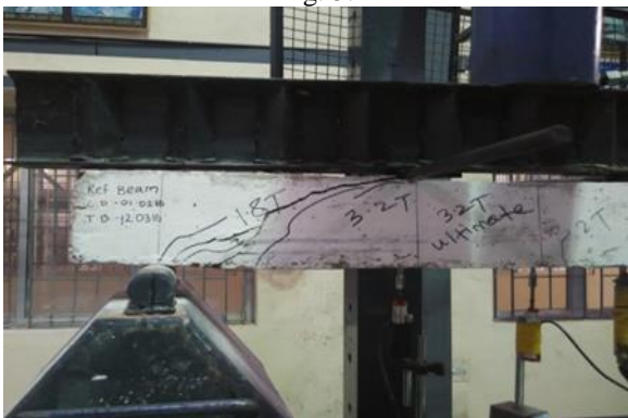
Fig. 4: Typical failure of reinforced concrete beam (control beam)
