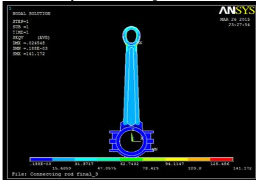
Fig. 7: Stresses and displacement of connecting rod in compressive loading condition
