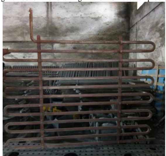
Fig. 3: Original Economizer tube front view
