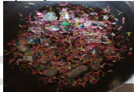
Fig. 2: Adding WPB to aggregate during heating
