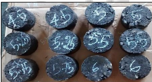
Fig. 1: Marshall Specimens for different bitumen %
