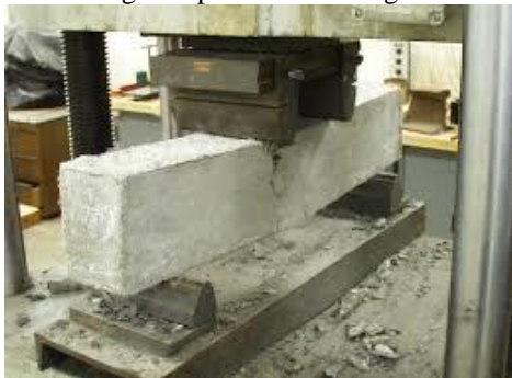
Fig. 4: Flexure set up
