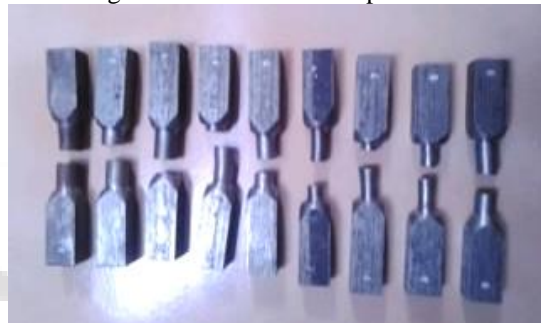
Fig. 2: Mild steel hollow specimens after failure
