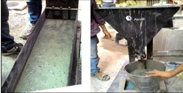
Fig. 3 Flow Ability In L-Box And V-Funnel Test
