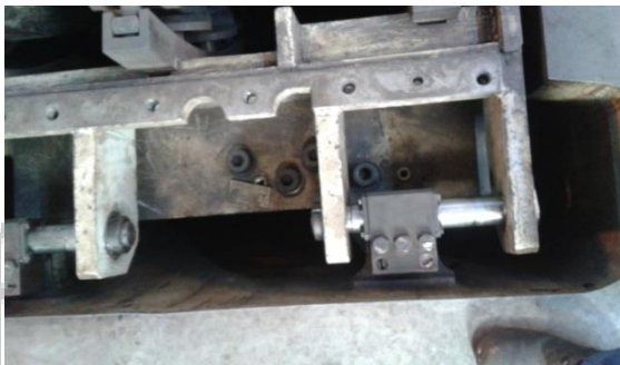
Fig. 6: Junction Plate Securing Pin
