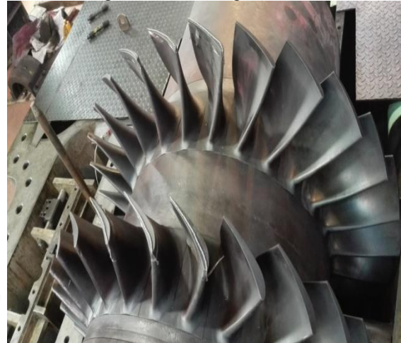
Fig. 5: cleaned turbine Rotor
