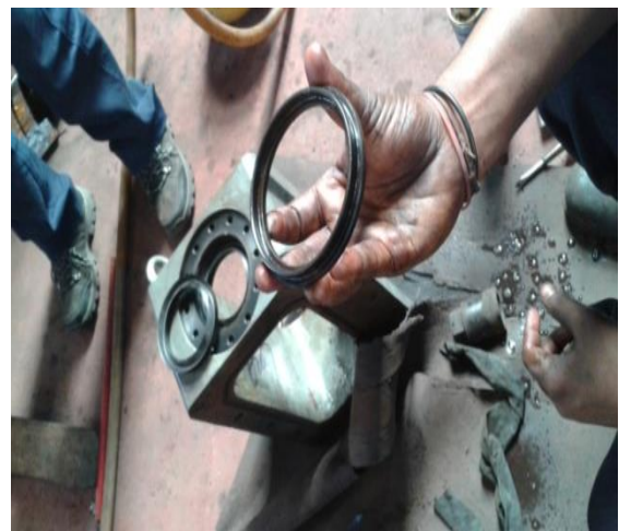
Fig. 5: Replacement of New Seals and Piston Rings
