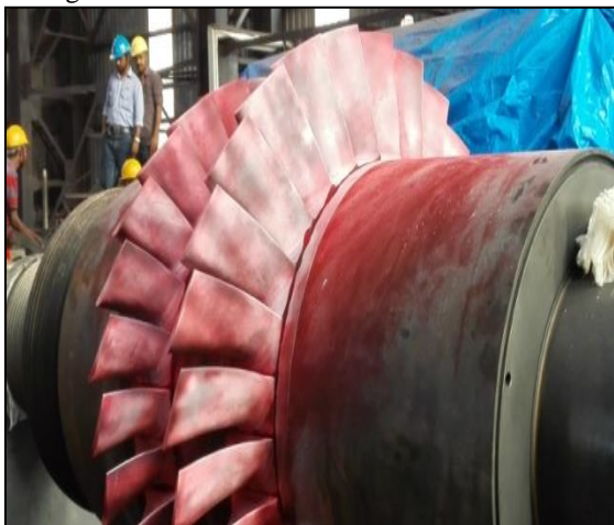
Fig. 3: NDT Testing of Rotor
